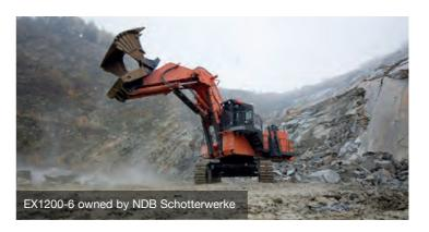
make gravel, chips and crushed sand. The two EX1200-6s are fitted with high buckets for excavating the granite and their excellent loading performance. "The Hitachi excavator was the most cost-effective solution we found," says NDB Schotterwerke's Managing Director. Peter Gusek.
