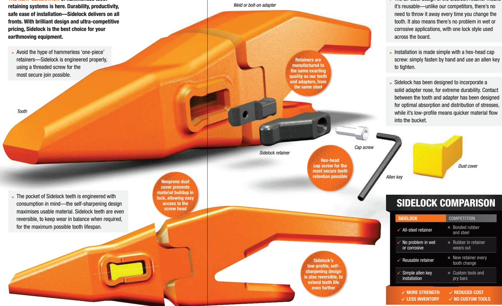
Weld or bolt-on adapter
