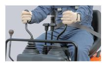
**Hydraulic Pilot Control Levers** Hydraulic pilot operation levers provide smooth control and easy operation.
