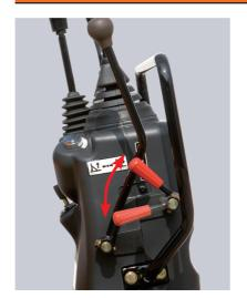
Lock Lever Allows Lock/Neutral Engine Starting
