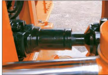
Universal joints are hermetically sealed to extend greasing intervals up to 12 000 hours, simplifying maintenance and increasing durability.
