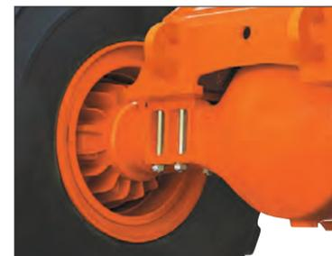
The outboard-mounted, sealed wet disc brakes produce plenty of braking force, and keep out dirt. Dual lines are independently provided for front and rear axles for added safety.
