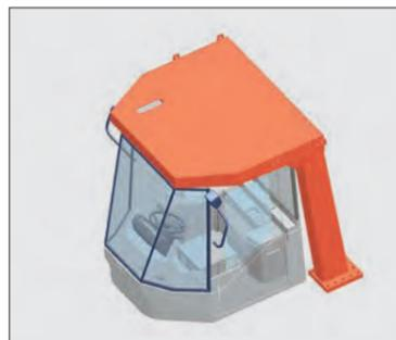
Outer ROPS/FOPS structure is adopted to protect the operator from injury in the case of an accident.
