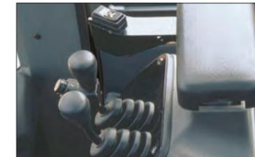
The directional switch is located next to control levers for easy travel direction changing. The operator does not need to left hand off the steering wheel.
