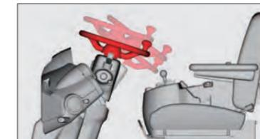
The steering column is tiltable and telescopic to suit operator's build for comfortable positioning and operation.
