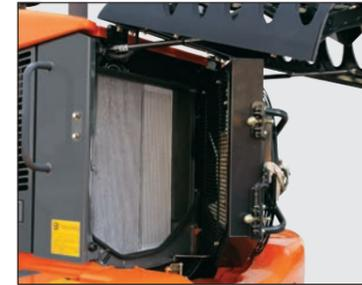
The radiator and oil cooler are made of aluminum instead of conventional steel or copper for corrosion prevention.
