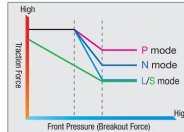
Traction force and front pressure are well balanced by work mode. If you need big traction force, select the P mode.
