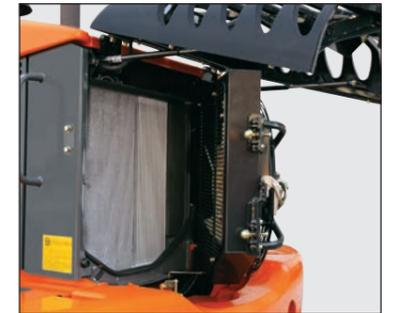
The rotation of the hydraulically operated cooling fan with heat-sensing system is equipped as standard. The fan itself can swing open for easy cleaning.
