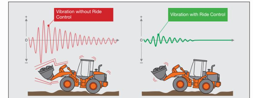
The ride control reduces pitching and bouncing during traveling on rough terrain and snow road by automatic control of the implement. Shocks and vibration can be well suppressed for riding comfort.
