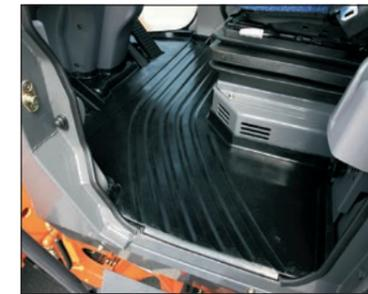
The cab floor is stepless (flat) for ease of cleaning.
