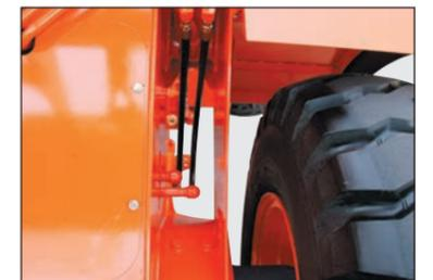
The DL front frame is shaped for easy removal of dirt, stones and snow.
