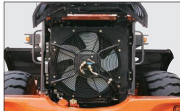
The cooling fan is enclosed by a full guard (metal net) to protect service technicians from injury during servicing and maintenance.
