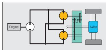
The two-motor HST system is newly developed to achieve high-efficient operation in a wide speed range. For instance, at a low speed, two motors yield high traction torque, while at a high speed, a single motor allows for high travel speed of 39 km/h. Moreover, this system makes possible easy slope climbing and smooth acceleration/deceleration with the accelerator pedal only.
