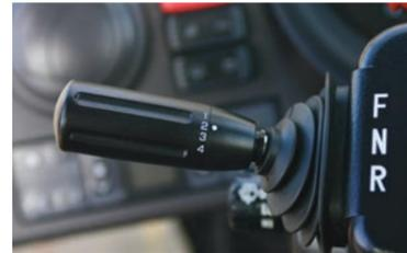
The fully automatic HST system is utilized for the selection of four maximum speeds according to job needs. Optimum speed can be selected with less shocks for smooth travel.
