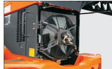
Fan speed can be adjusted depending on fluid temperature to effectively cool down coolant and hydraulic oil. The result is extended component service life and reduction in fuel consumption. The fan is also separate from the engine for easy servicing.
