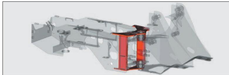
The box-section frame is thickened and strengthened to resist torsion and increase durability. Center pins are widely spaced for higher resistance to torsion.
