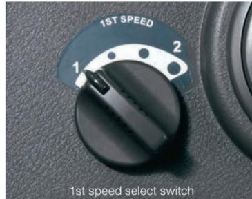
When the first speed range is selected, four travel speeds can be further selected to suit job needs and jobsite conditions. No need for skilful control of the accelerator and brake.
