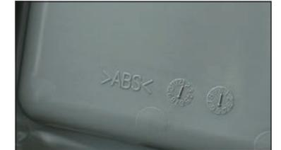
Approximately 95% of the ZW Series can be recycled. The resin parts are marked to facilitate recycling. The machine is completely lead-free. The radiator and oil cooler are made from aluminum and all wires are lead-less. In addition, bio-degradable hydraulic oil is available for jobsites where special environmental care is required.
