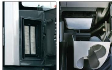
The fresh air filter can easily be replaced from the cab, and circulation air filter also replaced by detaching the drink holder.
