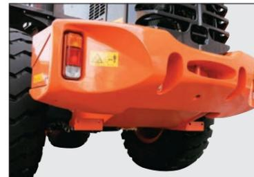
The large counterweight is arranged to protect the fuel tank from collisions with obstacles during operation.
