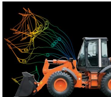
With the parallel/tandem hydraulic circuit, the lift arm and bucket can be operated simultaneously. This is a new function to increase loading and excavating efficiency.
