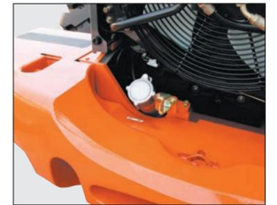
The fuel supply port is located for convenient fuel supply from the ground.
