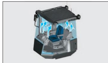
With the front and rear defrosters, airflow comes out from three front air outlets and two rear outlets to protect respective windows from fogging, keeping clear vision even in rain and cold weather.
