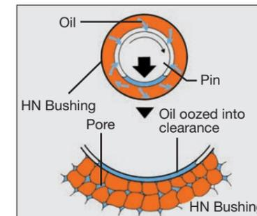
The HN bushing, another example of innovative technology developed by Hitachi, features long life and high durability. High-viscosity oil is vacuum impregnated in sintered high-hardness metal. During operation oil oozes from the pores of the bushing into the clearance between pins and bushing providing lubrication.
