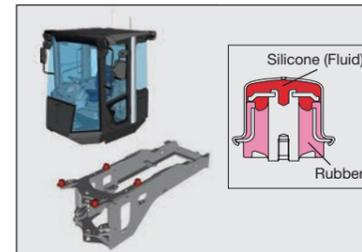
The cab rests on fluid-filled elastic mounts to absorb shocks and vibration, and reduce resonance.
