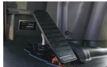
The operator can easily control travel speed with the inching pedal, regardless of the accelerator pedal, by adjusting the delivery flow from the hydraulic pump. This eases positioning in loading operation.
