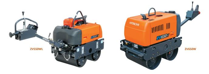
The ZV-W Series is designed for high performance in tight urban spaces, making it ideal for confined work sites. Equipped with a 4.0 kW engine, it delivers consistent power while maintaining fuel efficiency, meeting the demand for eco-friendly equipment. The ZV550WL features a 586 mm compaction width, while the ZV650W offers 650 mm, both ensuring quick manoeuvrability and maximum coverage with fewer passes, enabling contractors to achieve efficient results with minimal downtime.
