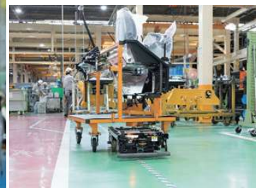
AGV(無人搬送車)の導入で、構内の一層の安全と省力化・効率化を図っています。 With the introduction of the automatic guided vehicle (AGV), we are working on further safety, labor saving, and efficiency improvements on the premises.
