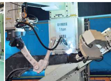
製缶部門では組み立て必要箇所に共用化治具、溶接ロボットを駆使して1個ずつ製作します。 In the can manufacturing process, we make full use of common jigs and welding robots in the order of assembly and manufacture cans one after another.
