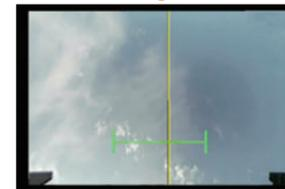
Before entering the trolley section, this function assists the operator in aligning the truck with the trolley line.
