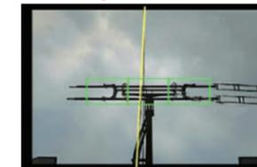
During trolley mode, this function assists the operator to drive within the contact range of the pantograph and trolley line.
