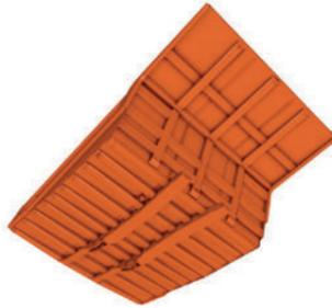
High strength 690 N/mm<sup>2</sup> (100 000 psi) alloy steel is also used for the canopy side members and floor stiffeners. The body is rubber cushioned on the frame.
