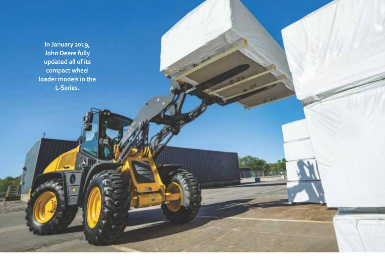
hydrostatic transmission with automatic shifting that has a top speed of approximately 23 to 25 mph [depending on the model]."
