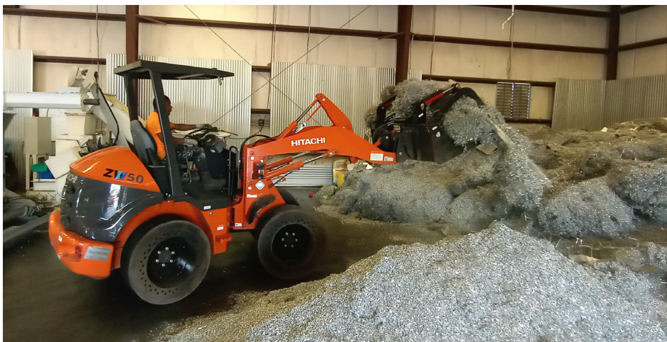
One of the most challenging jobs in the company is loading aluminum turnings. These are fine strands of aluminum that come off lathes and milling machines, and Pasco regularly receives and processes tons of it.
