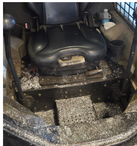
With a skid steer, aluminum shavings fell on the operator with each bucket-full.
