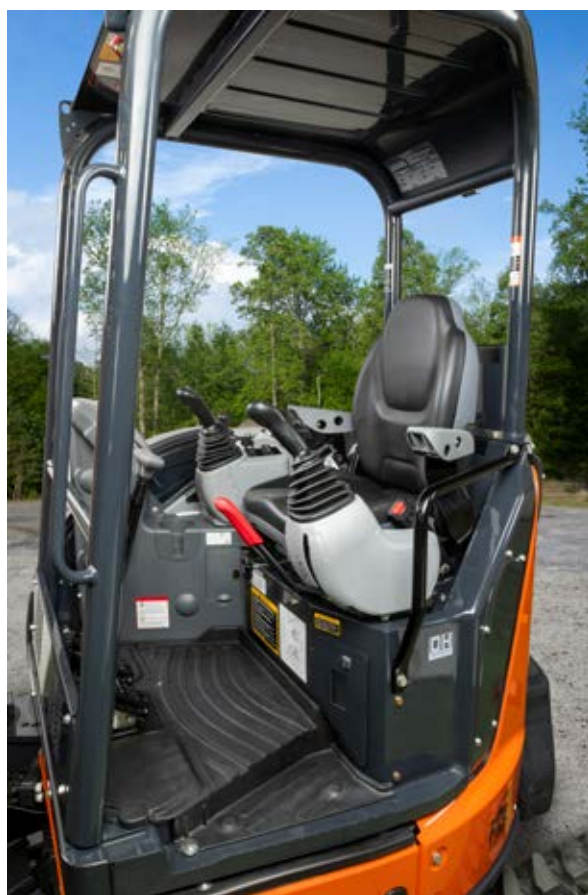
Above: Joystick controls for effortless operation and multi-function LCD eco-display makes operation easier.
