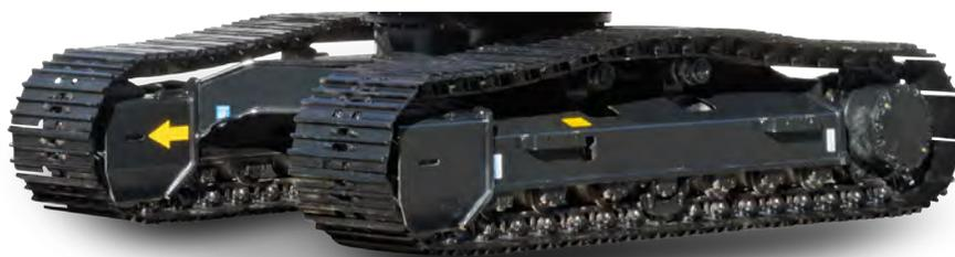
Reinforced undercarriage and increased crossbeam size and strength increase durability.
