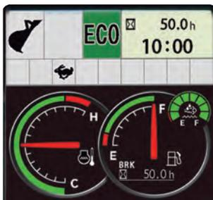
Checking DEF fluid level through Multi-function monitor.
