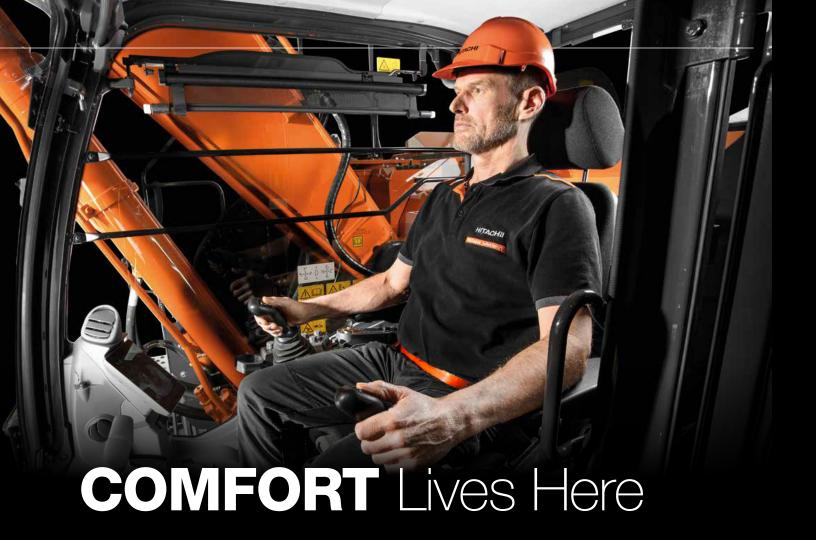
See and be seen: a larger interior with more head clearance and less noise, a panoramic view from the cab, and one-touch adjustable air suspension seat synchronized to move with the console. ROPS and FOPS certified cab.
