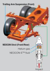
Each controlled by a hydraulic steering cylinder, rotates around the king-pin and the outer end of the trailing arm to position the wheels for steering. The spindles are attached by one simple tie-rod.
