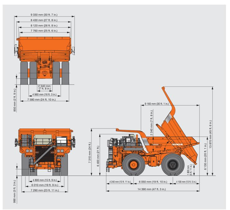
Note: Dimensions shown are for an empty machine with 46/90R57 tires. Exact dimensions may vary due to tire make, type, and inflation pressure
