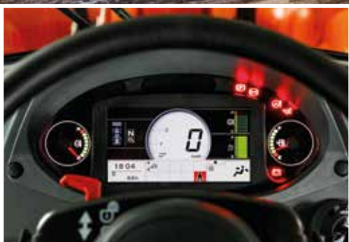
New LCD monitor shows the machine's status and settings.
