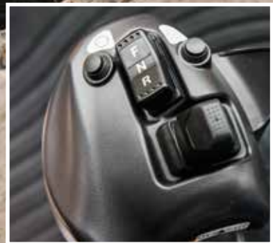
The optional e-Stick Steering System provides exceptional control.
