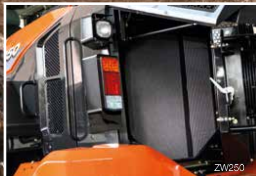
Optional clog resistant cooling cores enhance durability.
