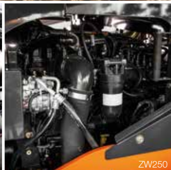
Tier 4 Final engine reduces fuel consumption.
