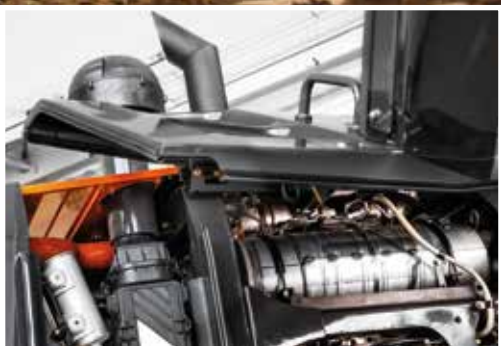
The SCR system reduces emissions.
