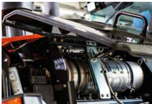
NO DPF SCR system reduces emissions.
