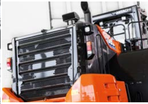
New rear grill protects radiator compartment.
