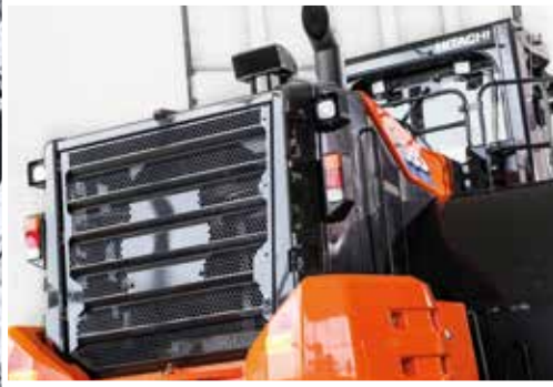
New rear grill protects radiator compartment.
