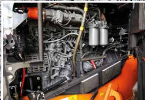
Tier 4 Final engine reduces fuel consumption.
