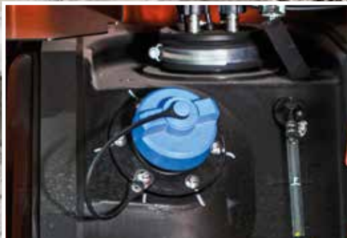
The urea tank is located for safe and easy access from ground level.
