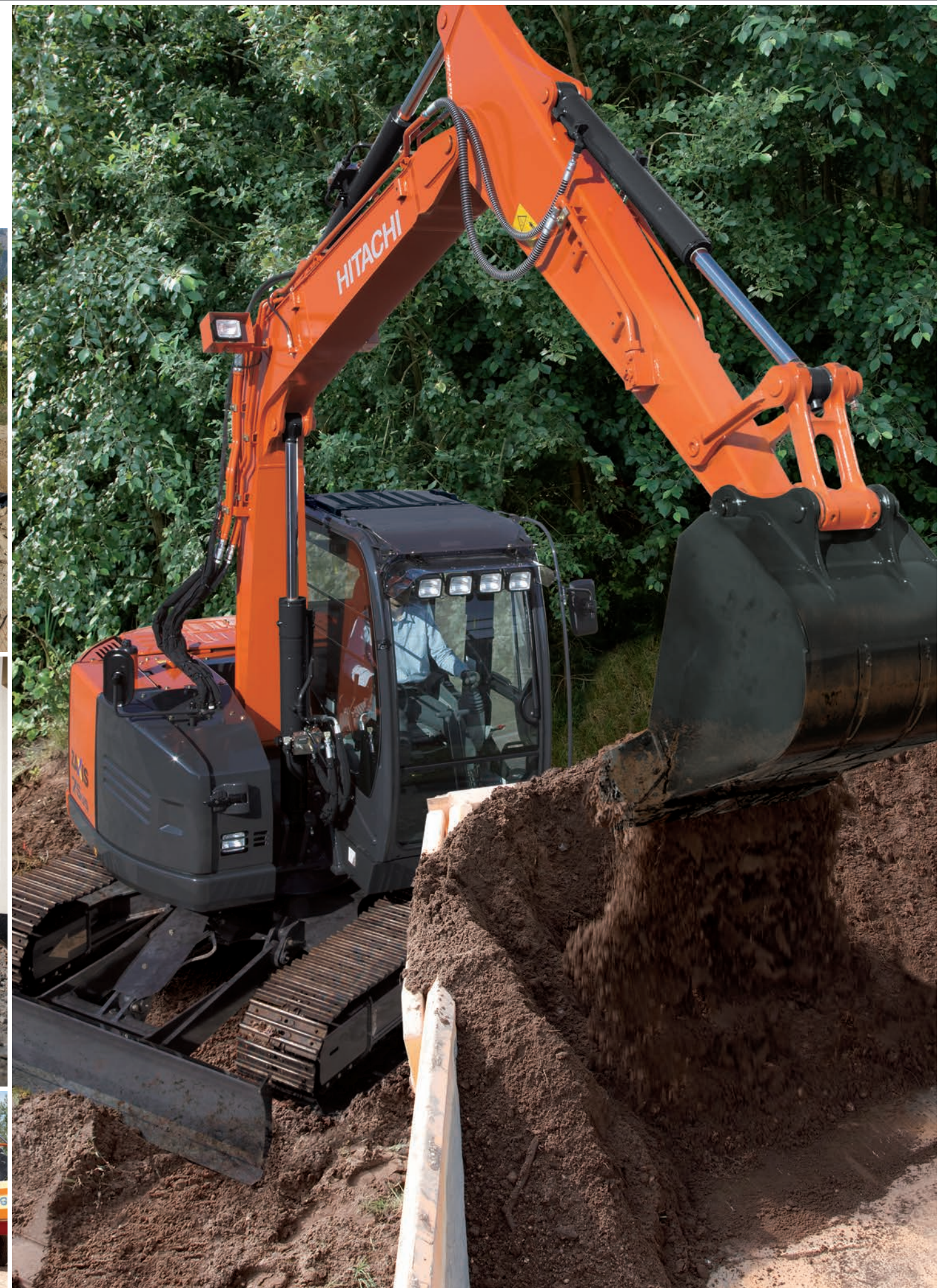
Shown equipped with 2.12m arm, extra piping, hose rupture valve, additional boom lights with cover, additional cab roof front lights, rain guard and rear view mirror and blade.
