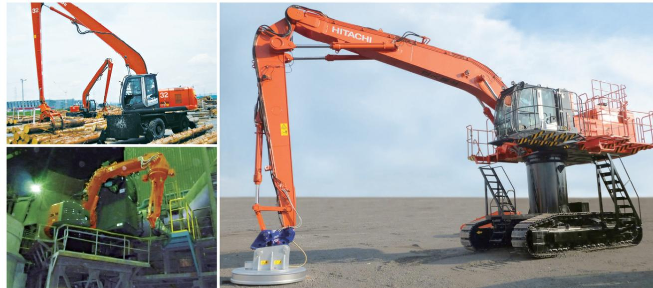
Customized products (application development) meet the individual needs of our customers. The ZX170WM-3 with log grapple comes with a dedicated grapple that simplifies the gripping a single thin piece of lumber (upper left). The ZX75US-3 with electric ladle dismantler has a rotating arm that makes it possible to remove slag from every corner of the pot (lower left). The ZX450LC-3 with high post materials handler secures a wide perimeter for working and offers favorable visibility (right).
