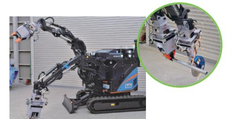
ASTACO-SoRa can handle a wide range of tasks by switching the tools attached to the end of its arms. The remote control has a numerous functions that assist the operator and offers a high level of operability.
