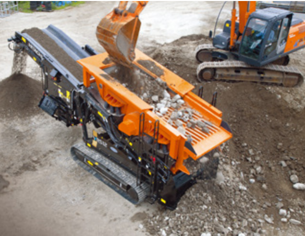
Track Mounted screen can be used to sort and process earth and soil at the scene of a disaster.
