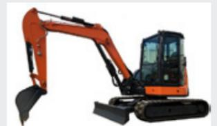
Prototype of battery-powered mini excavator
