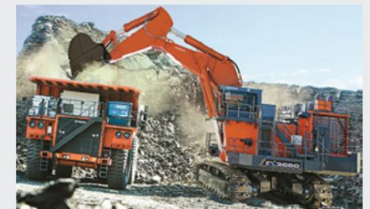
The EX3600-7 ultra-large hydraulic excavator (at right) that will be used in the verification tests
