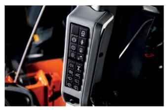
All commonly used functions can be selected at a glance using the side panel switch.
