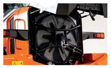
Intelligent fan operation system prevents radiators clogging.
